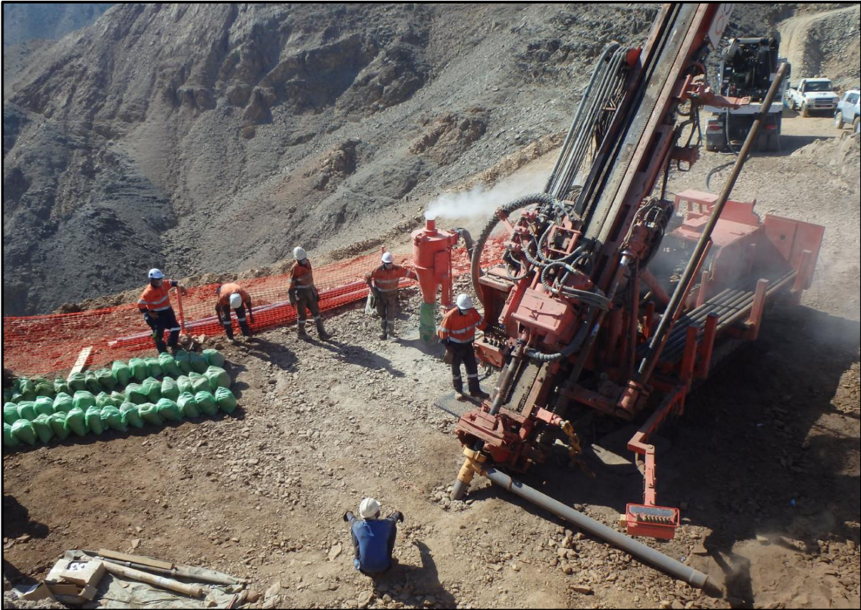
Figure 1: Capital Drilling's Gemrok MP-1000 multi-purpose rig #256 drilling on hole ROP-001 at Aladdin's Hill
