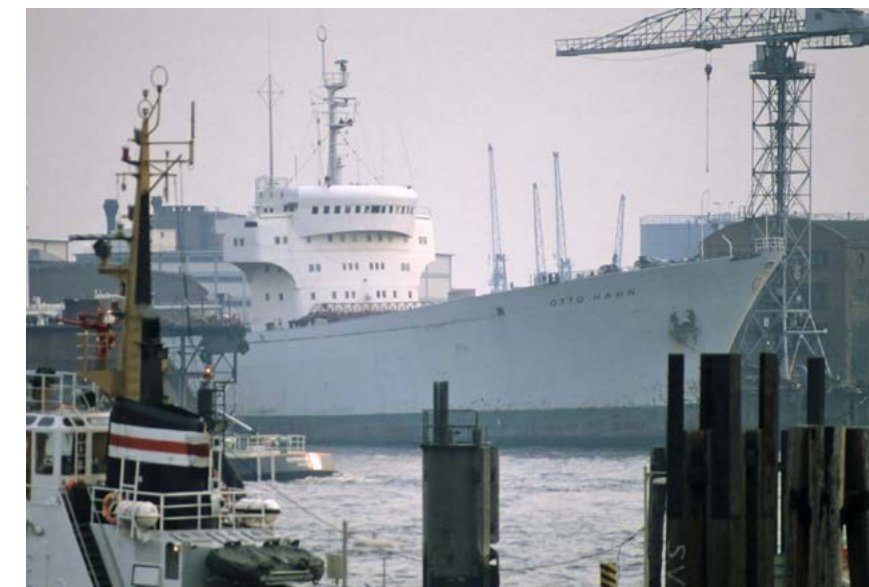
Otto Hahn was one of three experimental merchant ships that were equipped with nuclear propulsion
