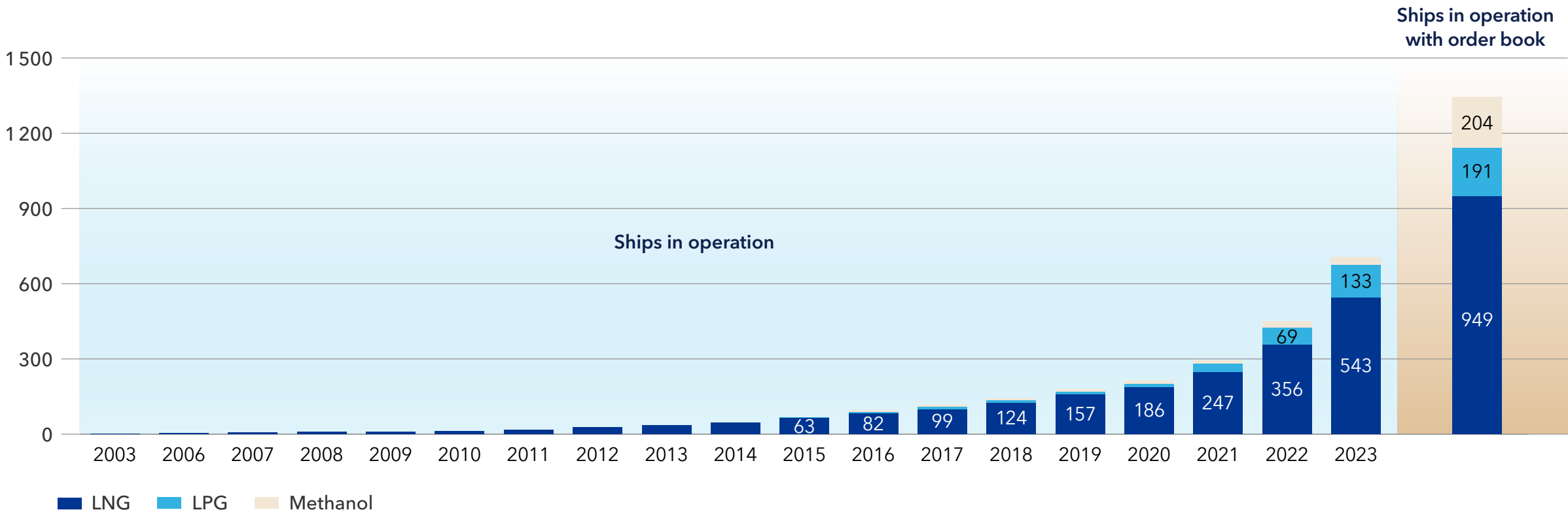
FIGURE 4-3 Development of LNG, LPG and methanol fuel technology uptake by number of ships, excluding gas carriers 47
