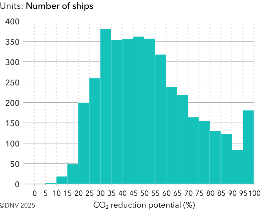
FIGURE 7-4 Number of containerships above 2 000 TEU (3 954 ships in total) with different annual CO 2 reduction potentials from onboard CO 2 capture, assuming given tank volumes and 100% capture rate
